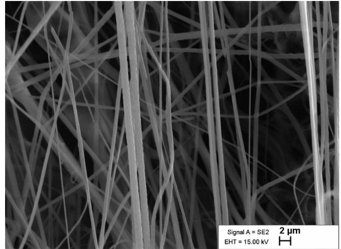
Figure 3. SEM image showing fiber diameter and distribution.
