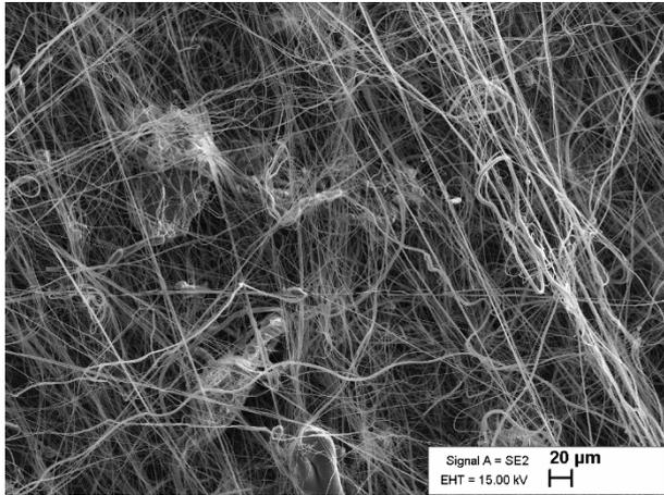
Figure 2. SEM image showing fiber morphology and porosity.
