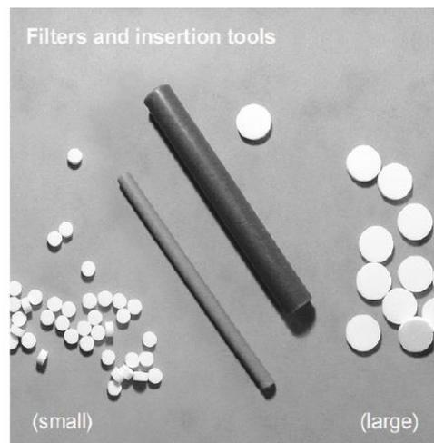
Small and large filters with different diameters (10  $\mu\text{m}$ , 35  $\mu\text{m}$  and 90  $\mu\text{m}$ ) are separately available, so you can use the filter of your choice.
