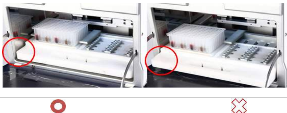
Figure 12. Correct and incorrect way of inserting plate on heating tray in the device
