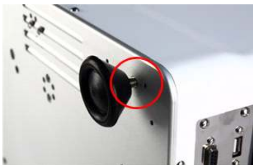
Figure 4. Adjust horizontality by turning the rubber feet (bottom view)
